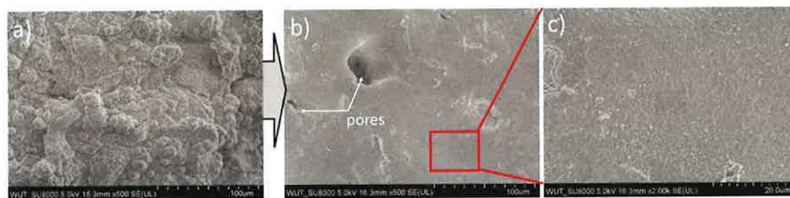
Fig. 12. Characterization of corroded surfaces of the LPBF-printed Mg-7.5Li-3Al-Zn alloy after 1 h of immersion in 0.01 M NaCl: a) surface covered with corrosion products, b) surface without corrosion products, c) surface without corrosion products shown at higher magnification.
